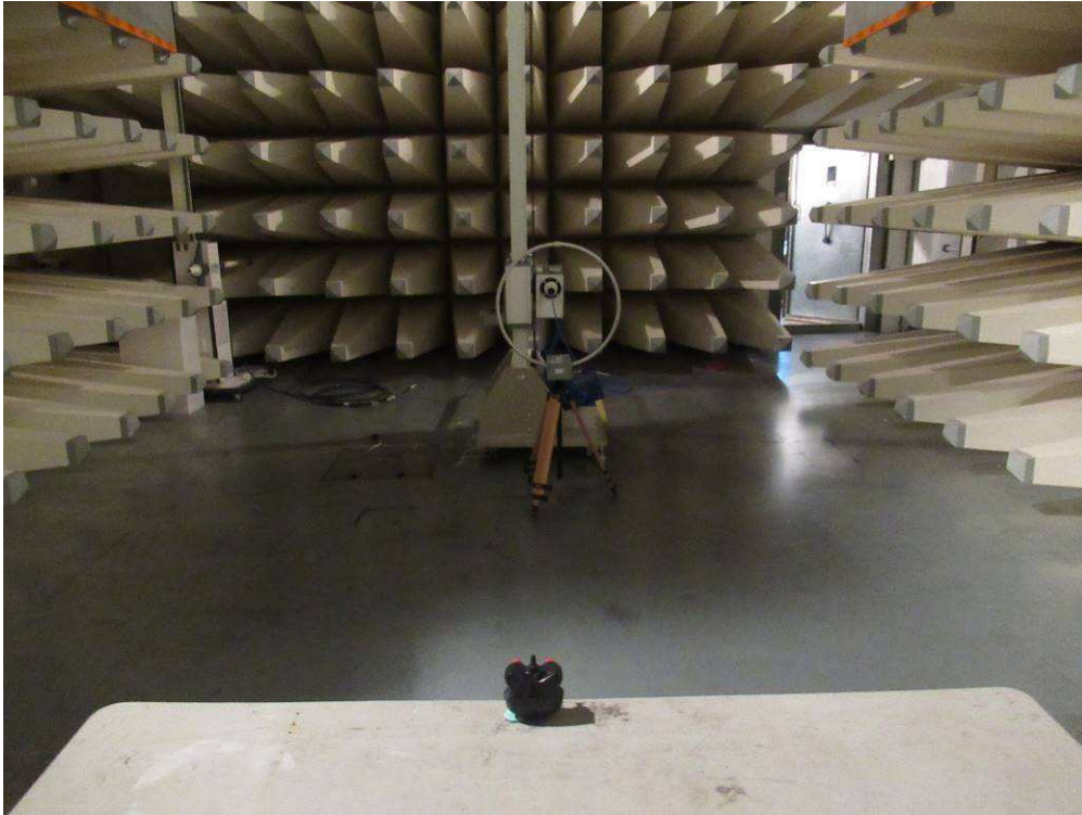
Setup for Radiated Emissions
