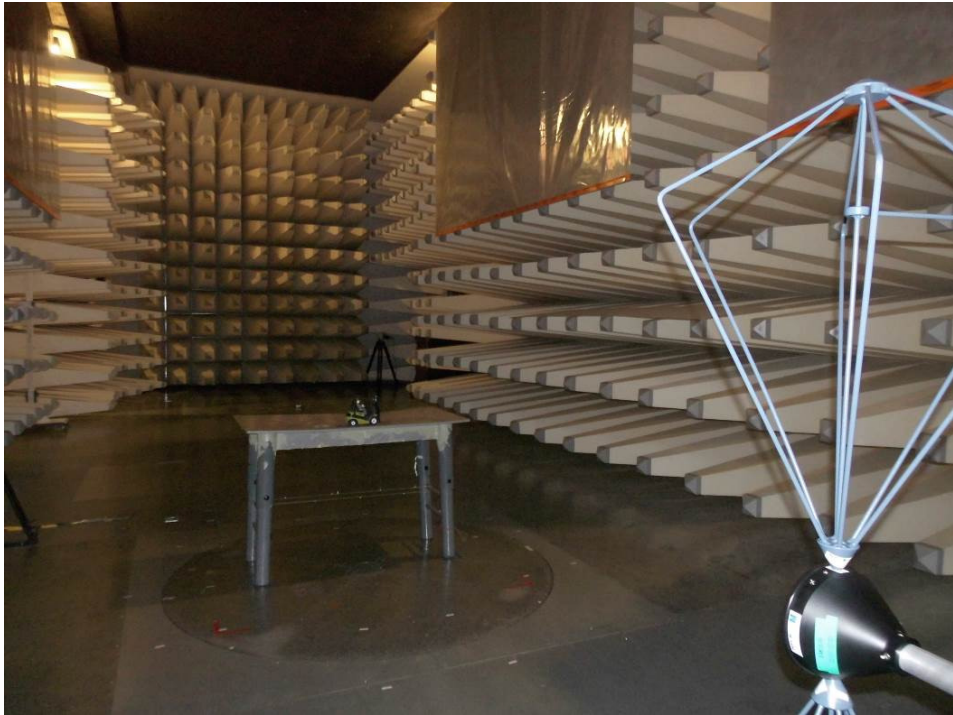
Setup for radiated emission
