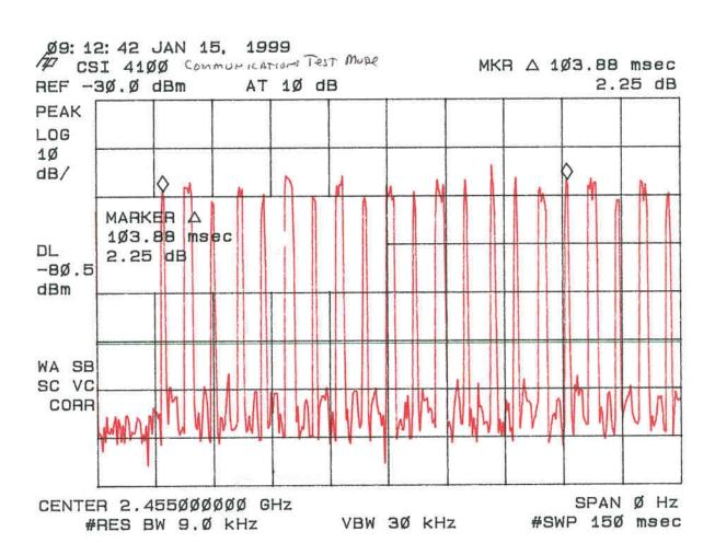
Figure 6d Duty Cycle Correction (Communications Test Mode)
