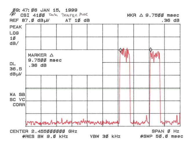
Figure 6c Duty Cycle Correction (Data Transfer Mode)
