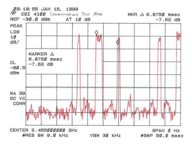
Figure 6f Duty Cycle Correction (Communications Test Mode)
