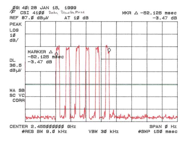
Figure 6b Duty Cycle Correction (Data Transfer Mode)
