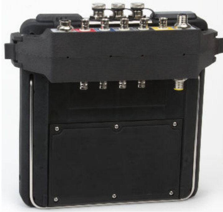
Figure 2-8: CSI 2140 Four-Channel Input Adapter attached to the CSI 2140 without the interface cable
