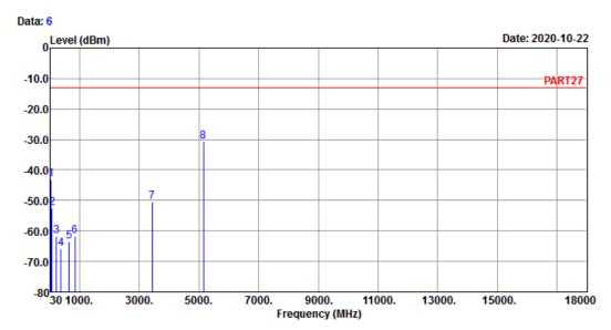
Site : 966 Chamber 5 Condition: PART27 VERTICAL Remak : 11N\_HT40\_TX\_CH38+
