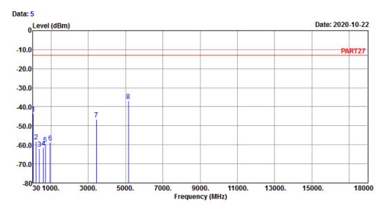
Site : 966 Chamber 5 Condition: PART27 HORIZONTAL Remak : 11N\_HT40\_TX\_CH38+
