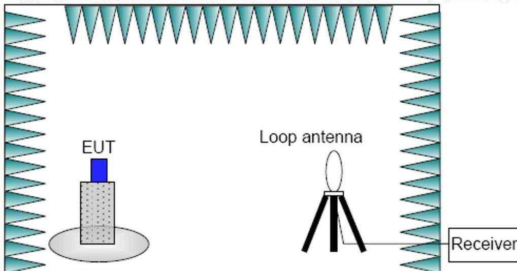
Below 1GHz Test Setup
