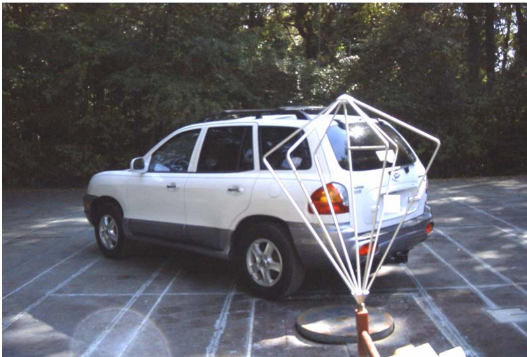
Lowest Margin for SLV1 radio in 2003 Hyundai Santa Fe is at 225 degrees
