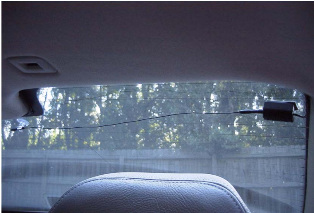
External remote antenna on 2005 Volvo S60
