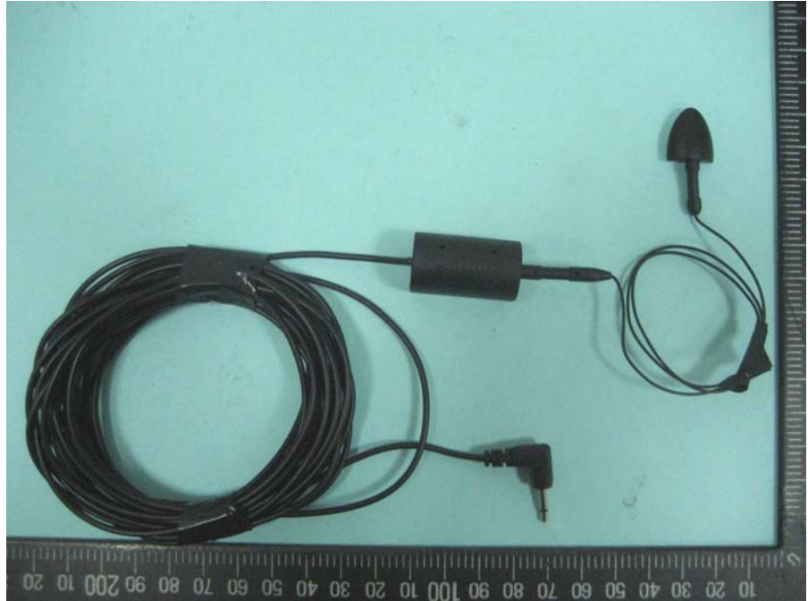
External FM transmitting antenna
