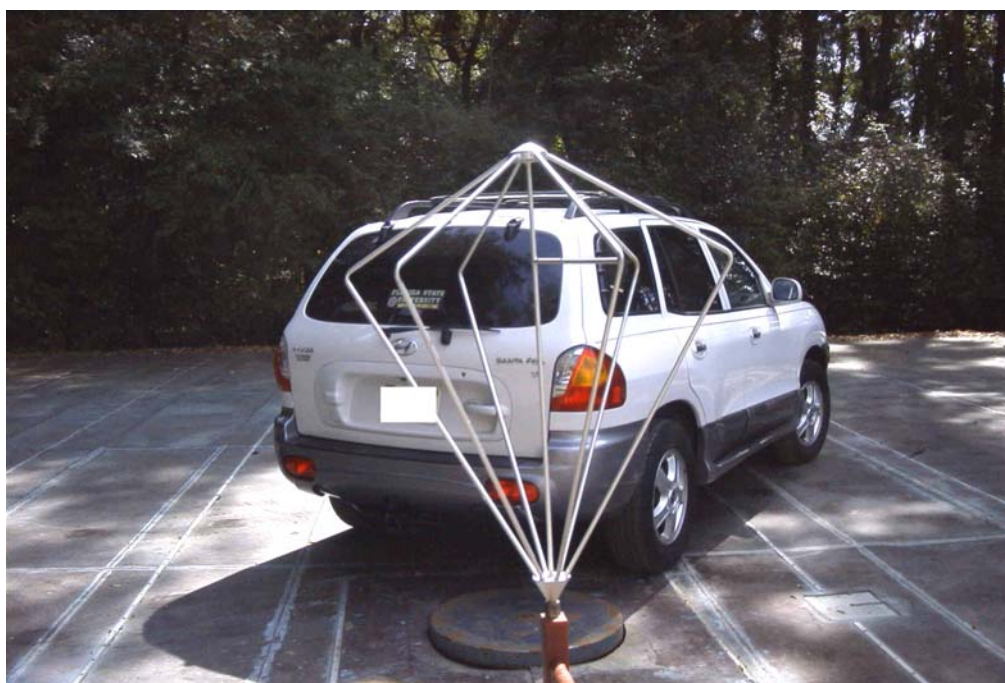
Lowest Margin for SV3 radio in 2003 Hyundai Santa Fe is at 135 degrees
