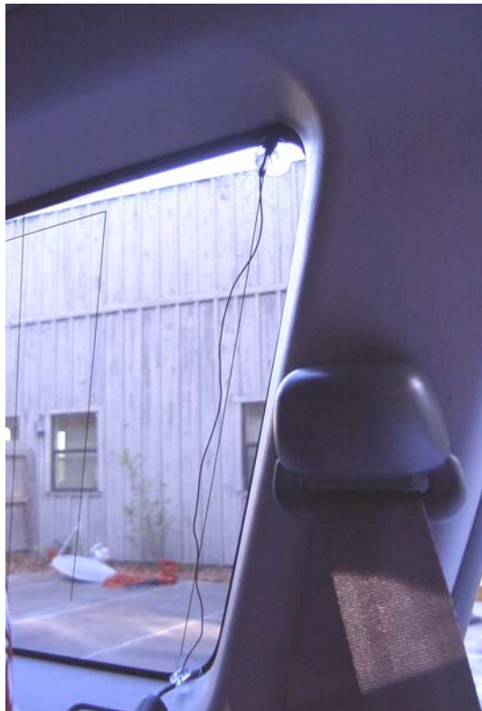
External remote antenna in 2003 Hyundai Santa Fe
