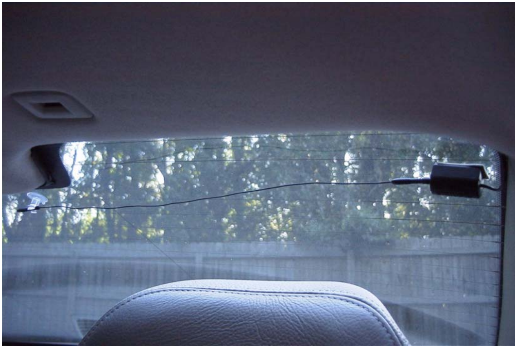
External remote antenna on 2005 Volvo S60
