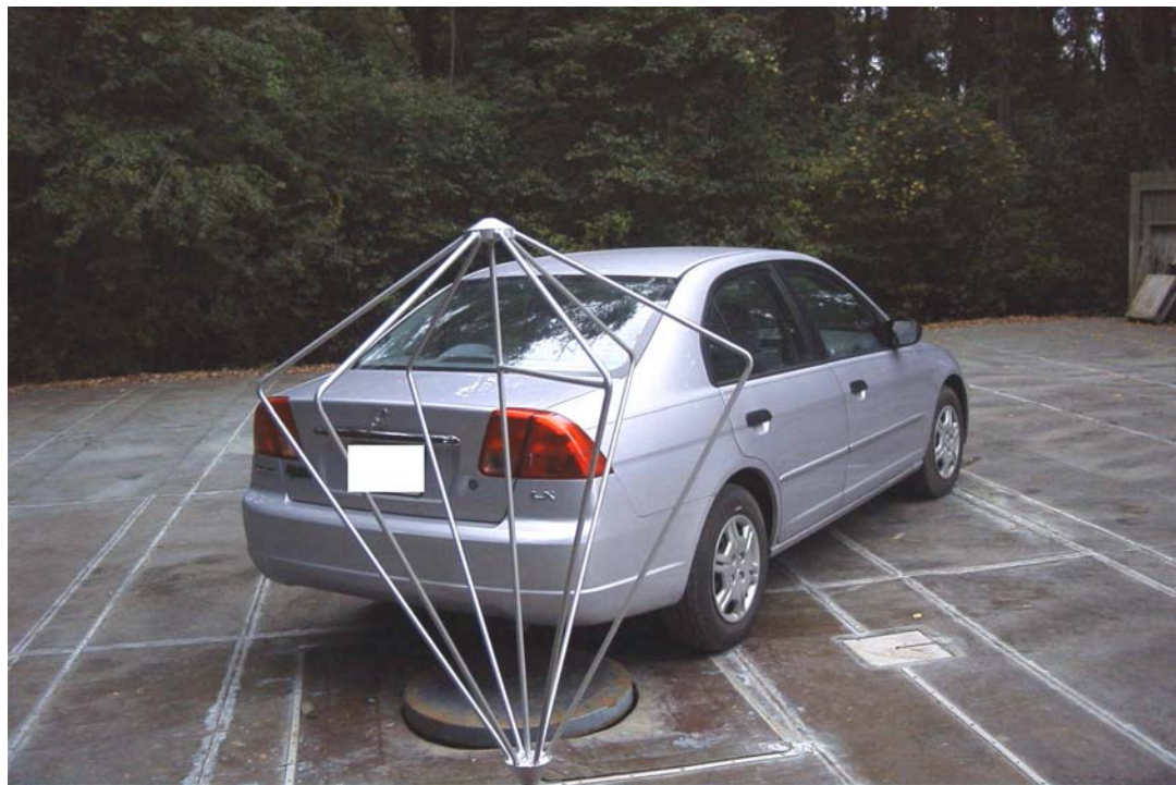
Lowest Margin for SV3 radio in 2001 Honda Civic is at 135 degrees
