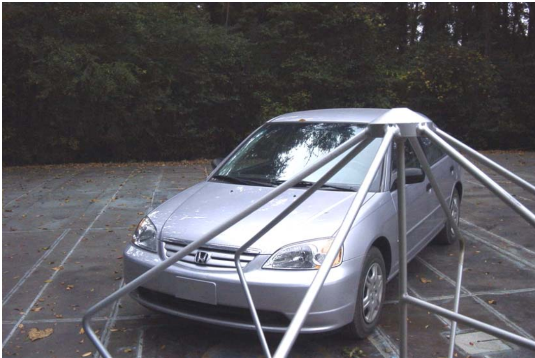
Lowest Margin for ST3/ST4 radio in 2001 Honda Civic is at 315 degrees
