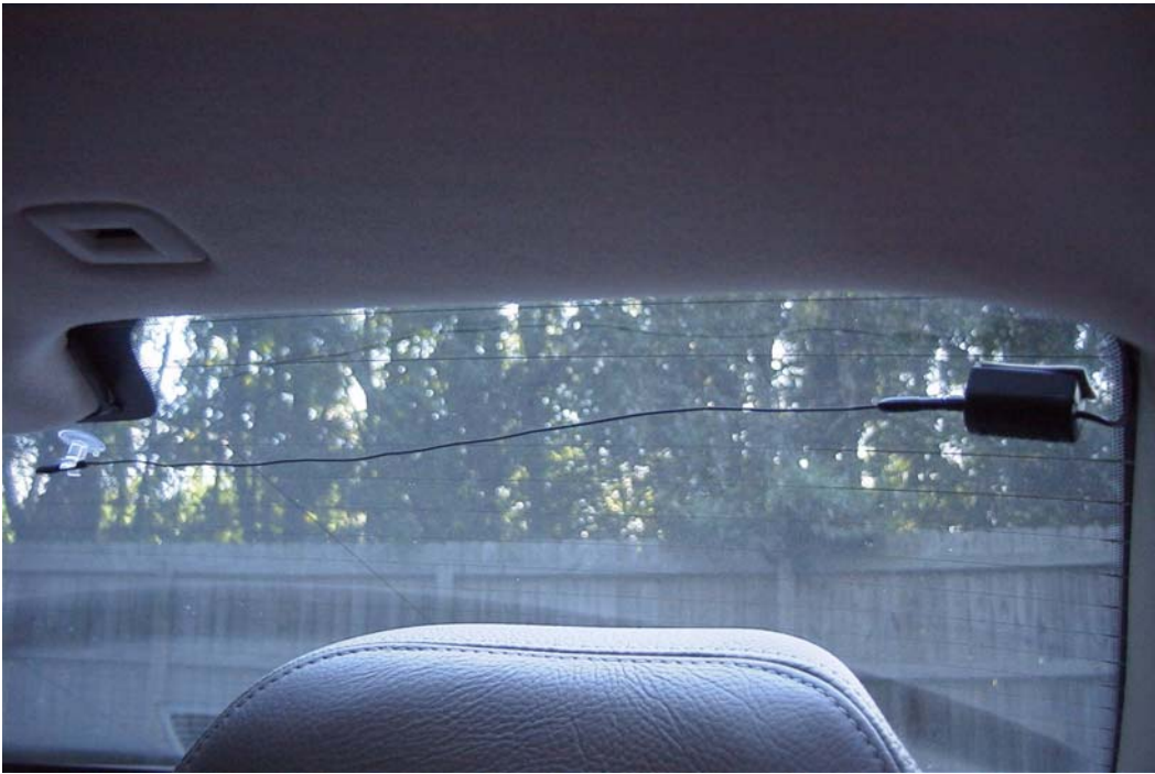
External remote antenna on 2005 Volvo S60
