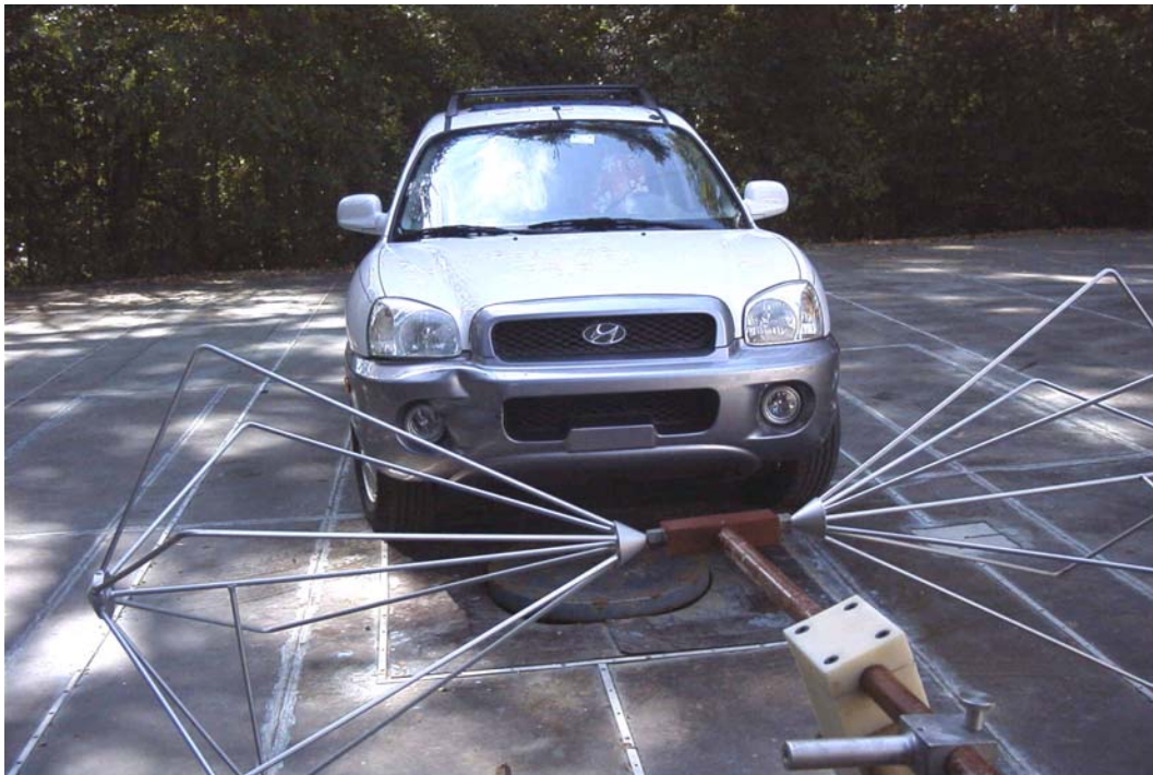
Lowest Margin for ST3/ST4 radio in 2003 Hyundai Santa Fe is at 0 degrees
