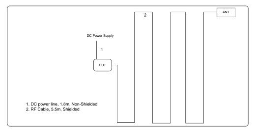
Note: The test configuration used in this testing produce worse emission nature.
