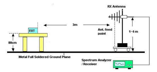
Above 10 GHz shall be extrapolated to the specified distance using an extrapolation factor of 20 dB/decade from 3m to 1.5m or 3m to 0.5m.
