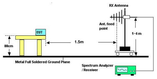
Above 10 GHz shall be extrapolated to the specified distance using an extrapolation factor of 20 dB/decade from 3m to 1.5m.
