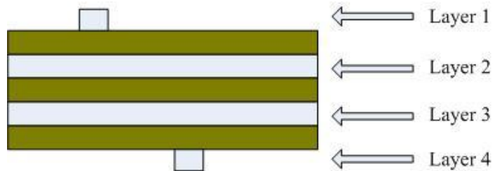
Figure 6-1-1-1 Application Board Layer Stack Up
