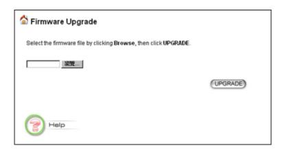
**Step 2:** To update the 802.11g Router firmware, first download the firmware from the distributor's web site to your local disk. Then from the above screen enter the path and filename of the firmware (or click **Browse** to select the path and filename of the firmware). Next, Click the **Upgrade** button.
