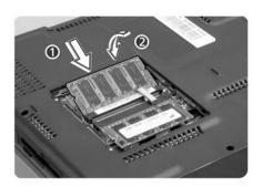
4 Replace the memory compartment door, and fasten the screw.
