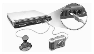
USB is plug and play, which means that you can connect and start using a USB device without having to restart your computer. You can also disconnect the device at any time.
