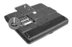
3 Insert the memory module diagonally in the slot (1), and then press down gently until it clicks in place (2).
