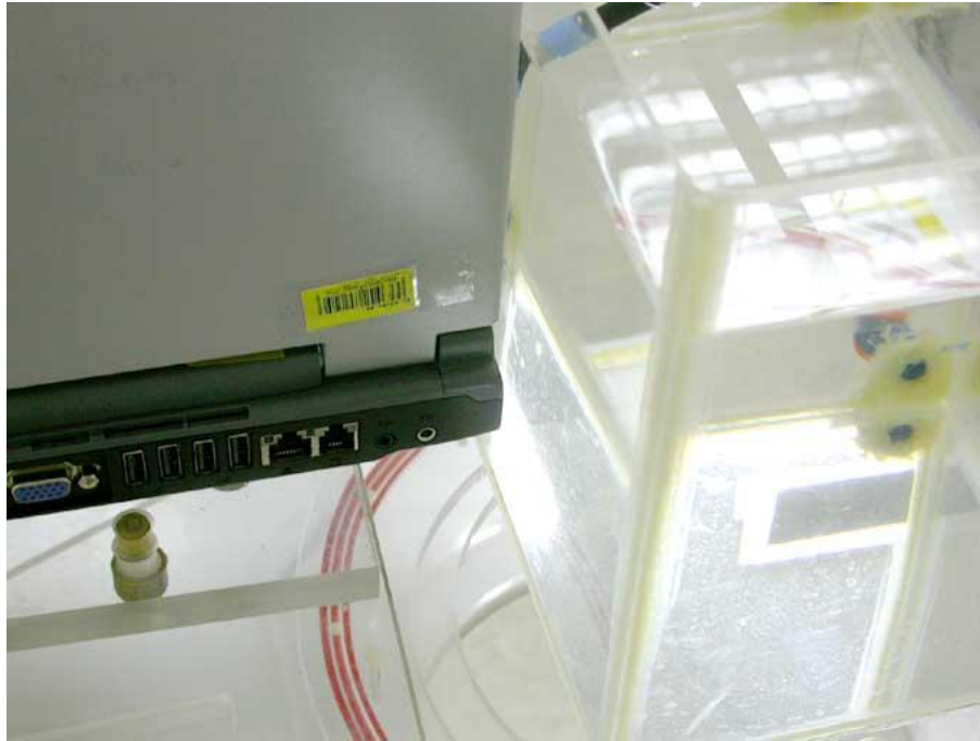
EUT perpendicular left to phantom - Zoom In
