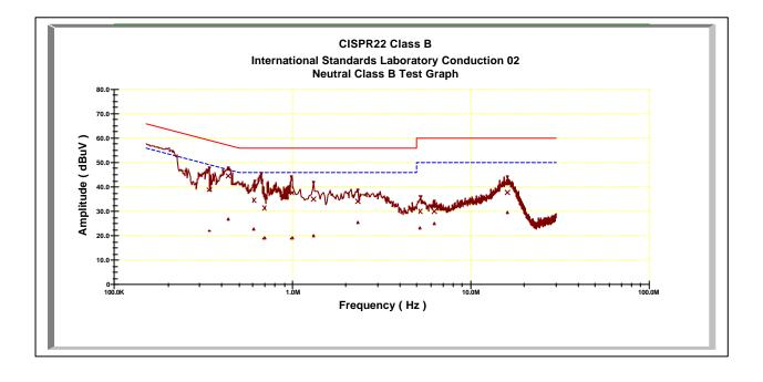
\* NOTE: During the test, the EMI receiver was set to Max. Hold then switch the EUT between Main antenna, Aux antenna Channel 1, 4, 5, 8, 9,12 of Normal
