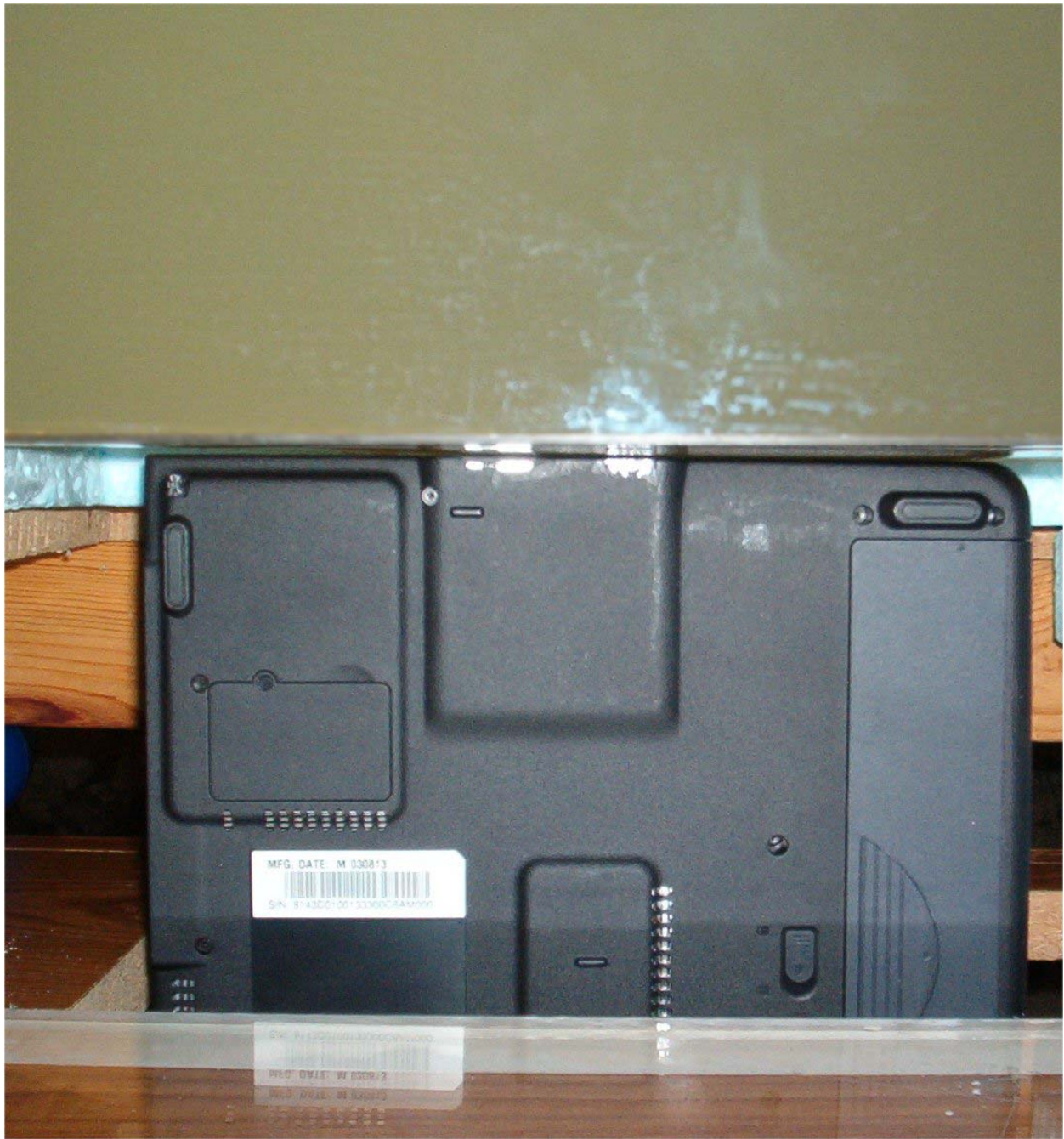
Fig. 3b. Photograph of the Acer Model MS2143 NoteBook Computer with left edge of the PC at 90° pressed against the base of the planar phantom. This is Configuration 2 for SAR testing and represents the case of a bystander in contact (at a distance of 0 cm) with the left edge of the PC.
