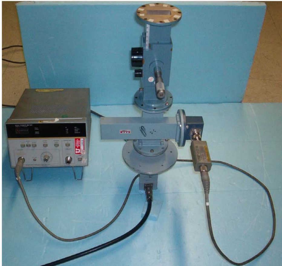
Fig. 1. Photograph of the rectangular waveguide radiator used for system validation. Also seen is the Narda Model 22CI movable slide screw tuner used to match the input power at 5.25 or 5.8 GHz to the planar tissue-simulant phantom.
