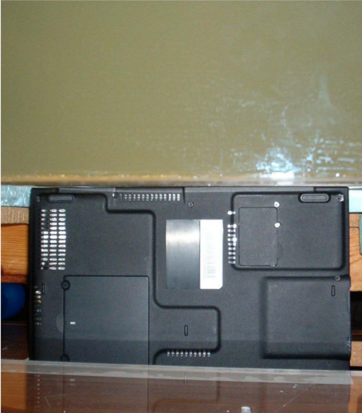
Fig. 4. Photograph of the Acer Model MS2143 Notebook Computer with the broader back edge of the PC at 90^\circ pressed against the bottom of the planar phantom with separation of 0 cm. This is Configuration 3 for SAR testing and represents the case of a bystander behind the PC screen with a separation of 0 cm.
