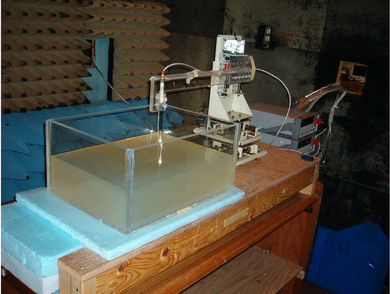
Fig. 5. Photograph of the three-dimensional stepper-motor-controlled SAR measurement system using a planar phantom.
