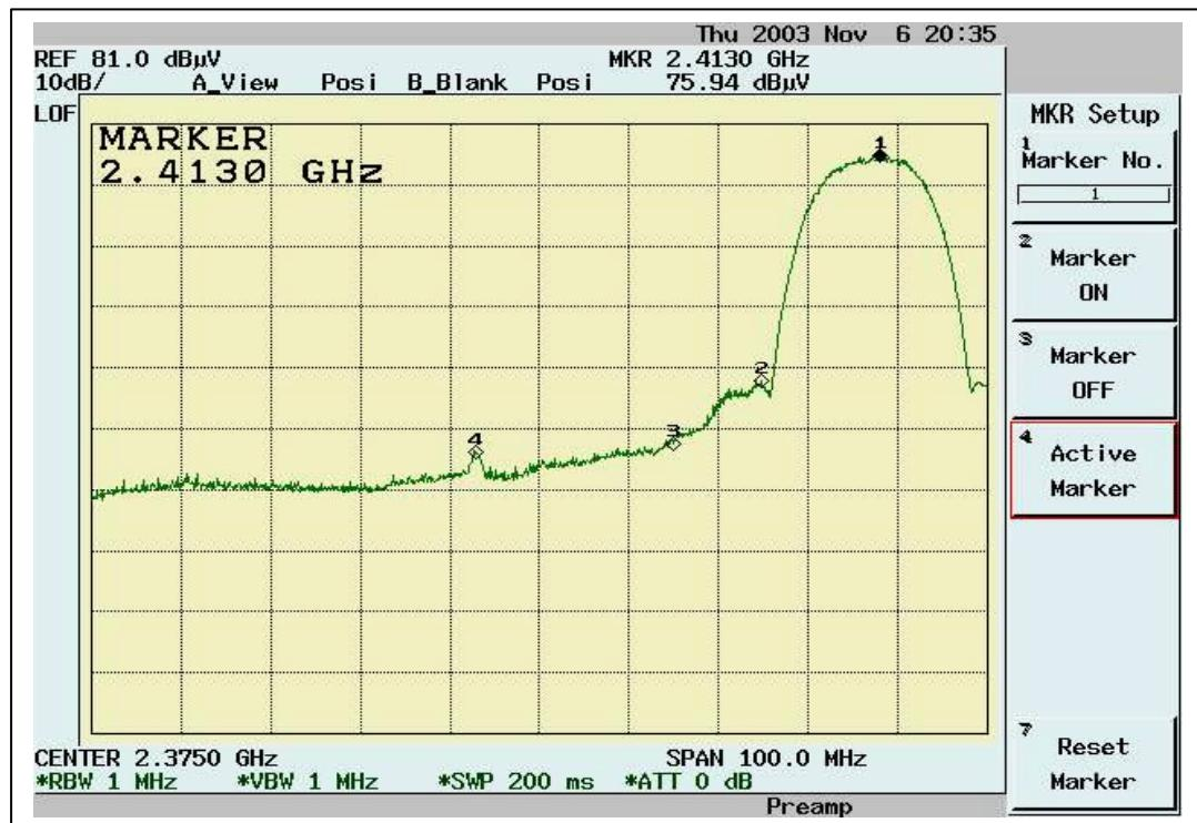
Band Edge measurement for radiated emission in Restricted Band(Radiated)
