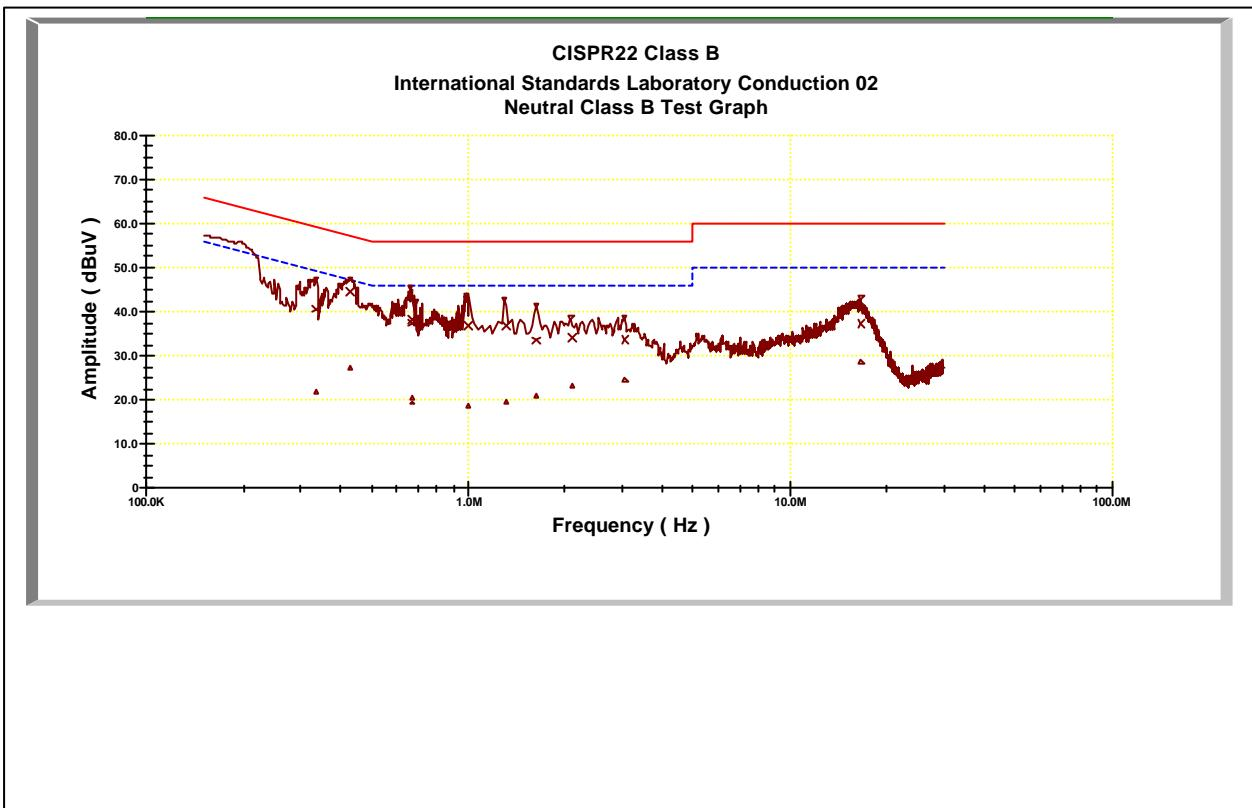
\* NOTE: During the test, the EMI receiver was set to Max. Hold then switch the EUT Channel between 1 , 6, 11 to get the maximum reading of all these channels .
