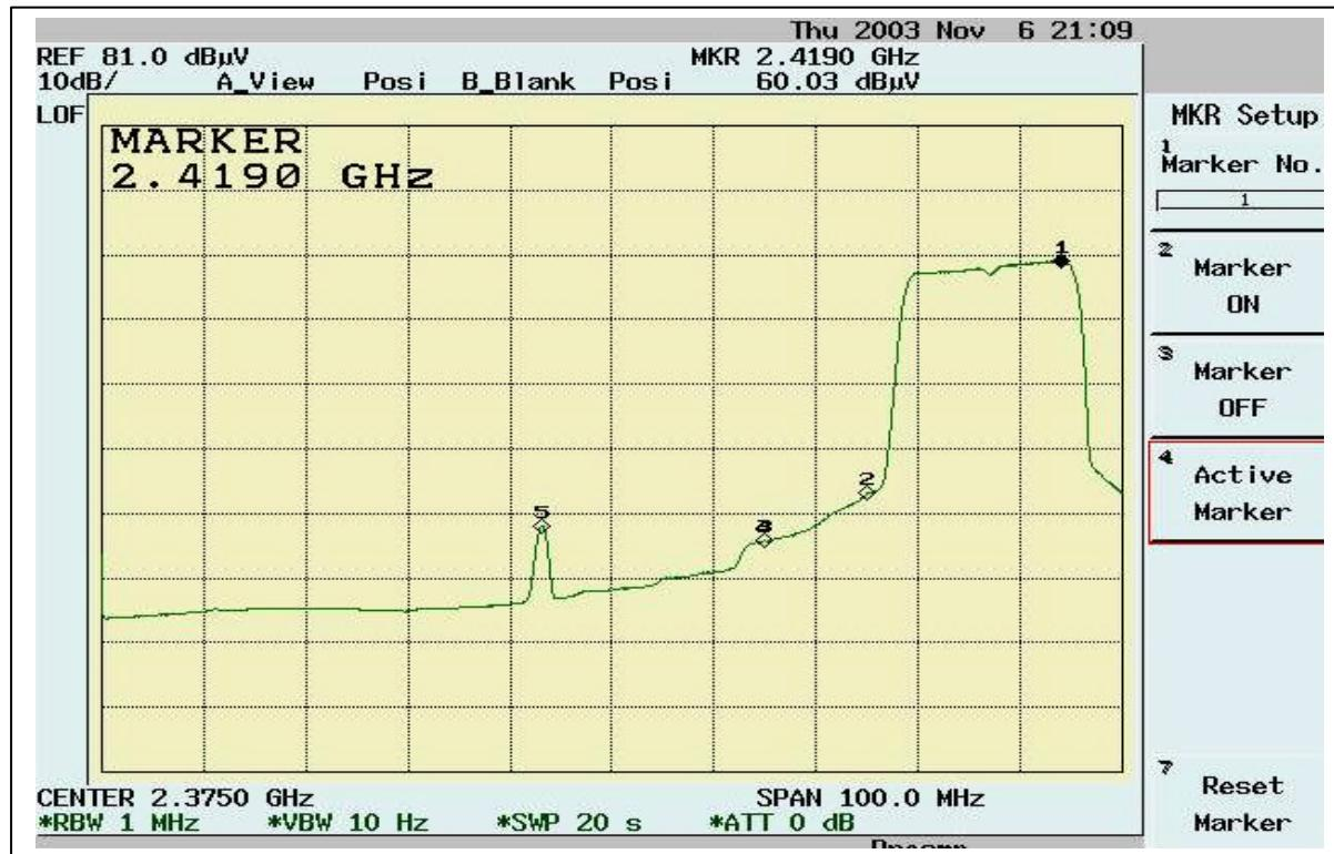
Band Edge measurement for radiated emission in Restricted Band(Radiated)
