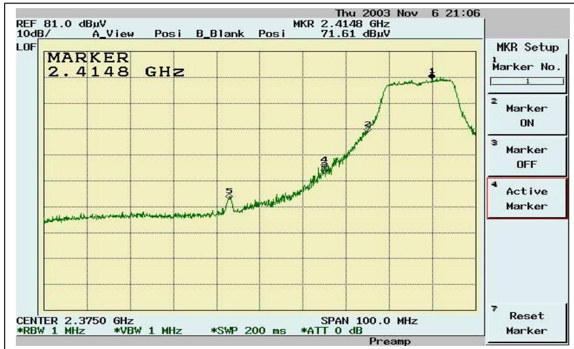
Band Edge measurement for radiated emission in Restricted Band(Radiated)
