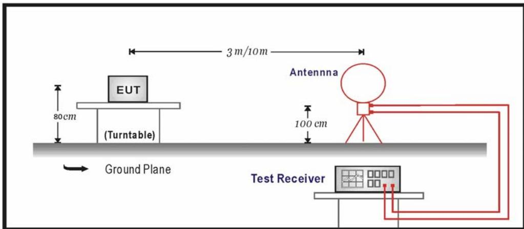
Under 1GHz Test Setup:
