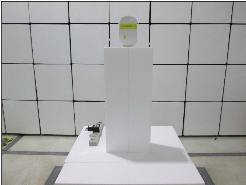
Radiated Emission Test above 1GHz
