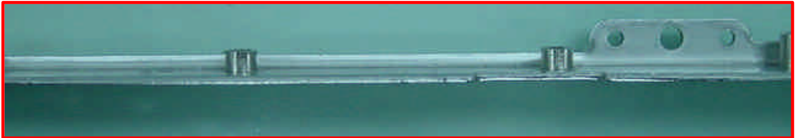
Cut down 1mm screw post height
