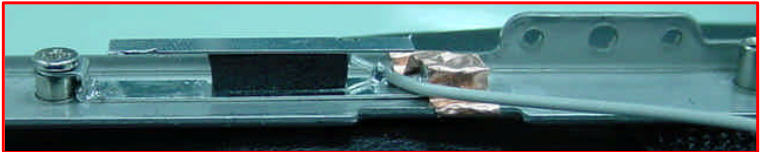
Cut down 1mm screw post antenna assembly
