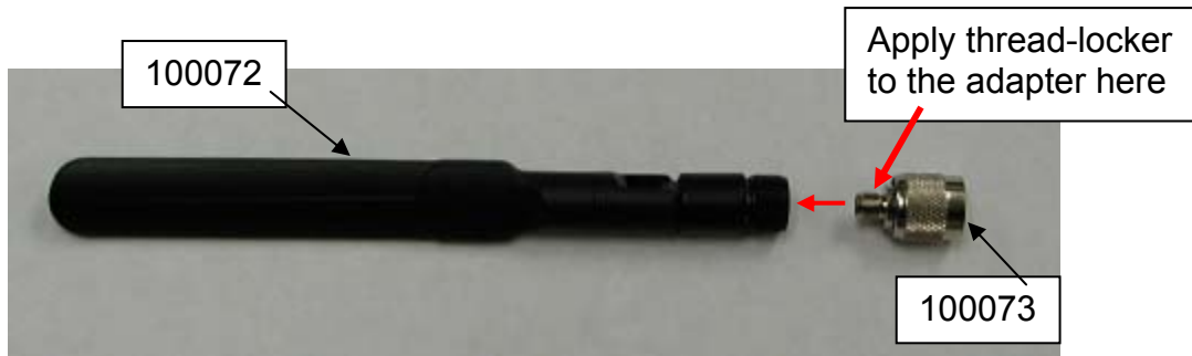
Figure 1. 70024 Assembly
