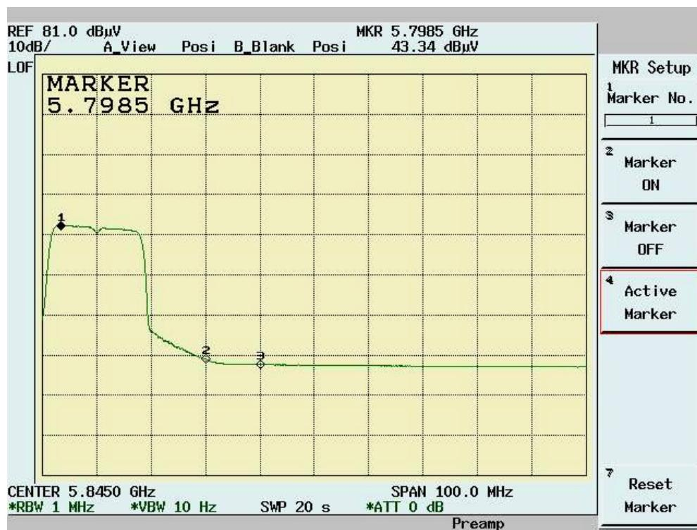
Band Edge measurement for radiated emission in Restricted Band(Radiated)
