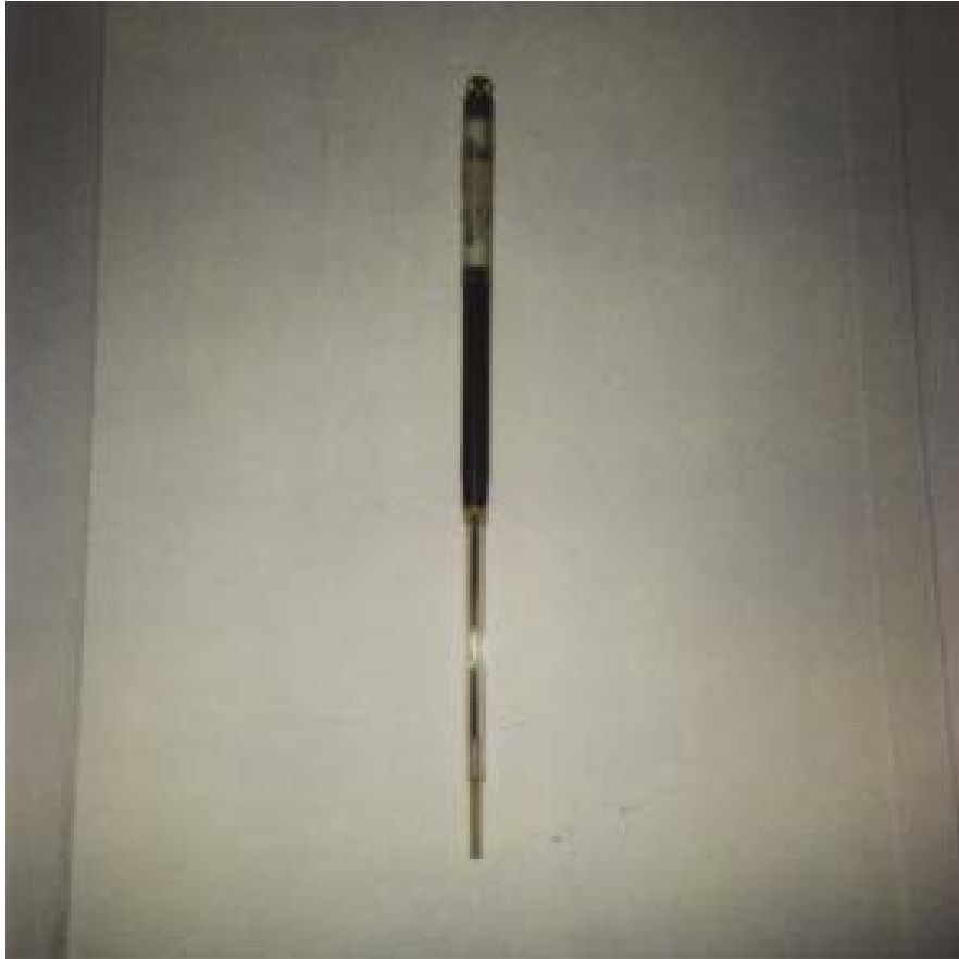
Fig. 11. Photograph of the Narda Model 8021 Broadband Electric Field Probe used for SAR measurements.
