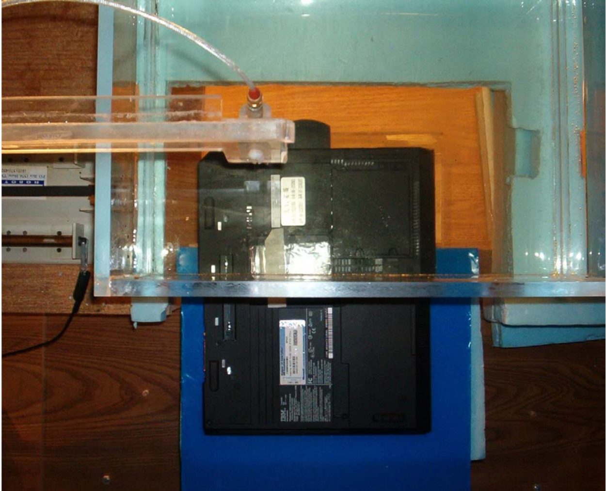
a. Bottom of IBM Model 2659-HT2 PC pressed against the base of the planar phantom.
