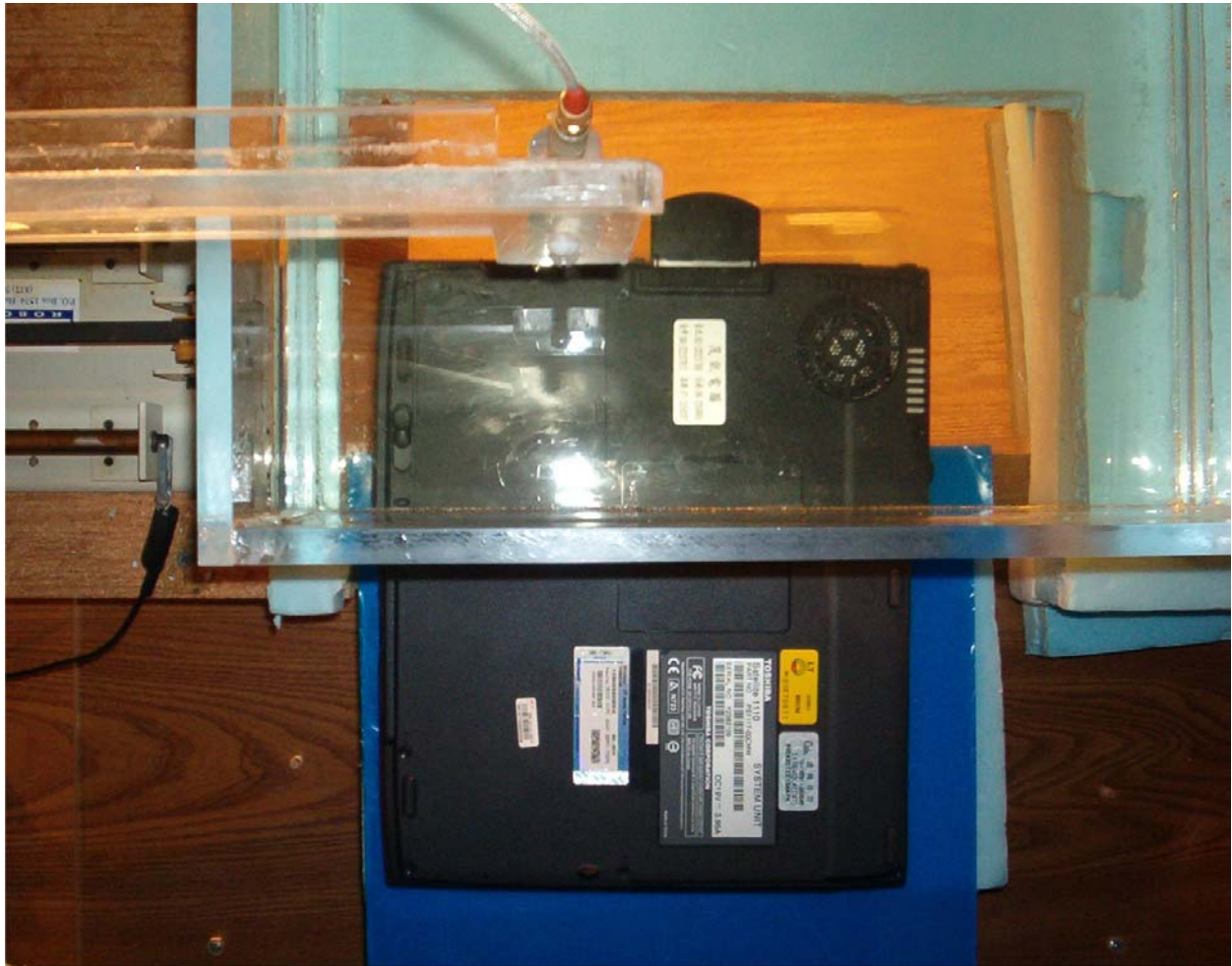
c. Bottom of Toshiba Satellite Model 1110 PC pressed against the base of the planar phantom.
