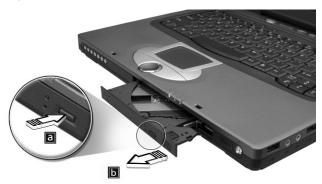
When the power is off, you can eject the drive tray using the emergency eject hole. See page 51.
