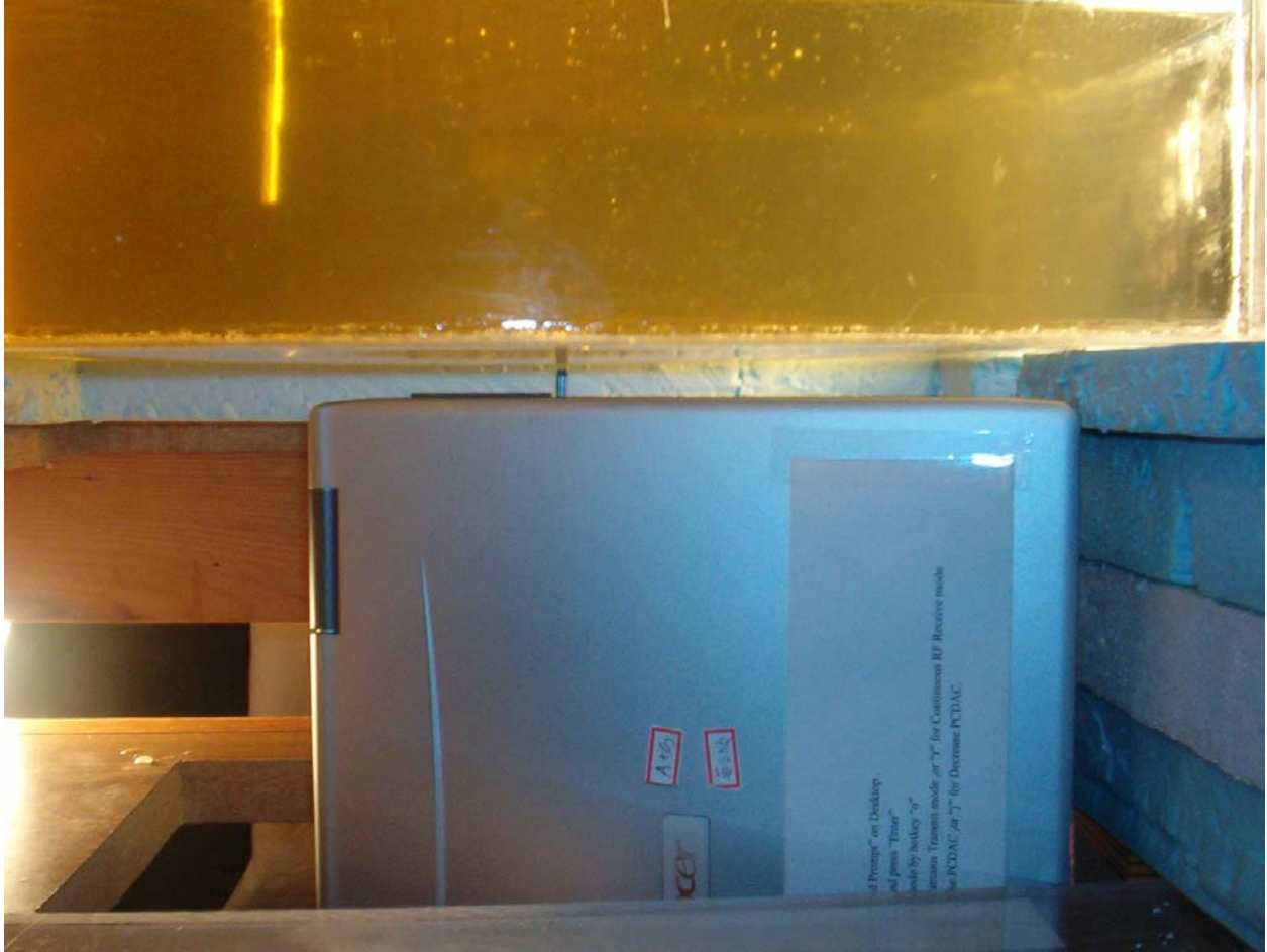
a1. Side view. The right edge with "Main" antenna at a distance of 1.5 cm from the bottom of the planar phantom.
