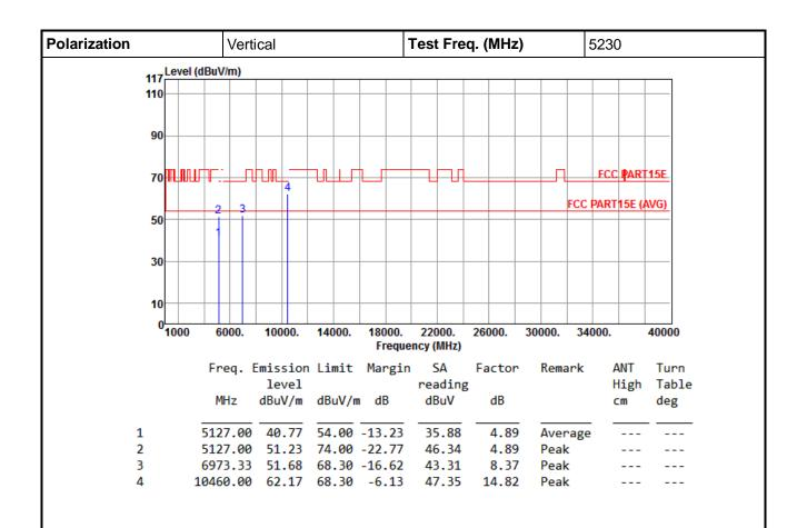
Note 1: ">20dB" means spurious emission levels that exceed the level of 20 dB below the applicable limit. Note 2: For restricted bands, the peak measurement is fully sufficient, as the max field strength as measured with the Peak-Detector meets the AV-Limit so that the AV level does not need to be reported in addition.
