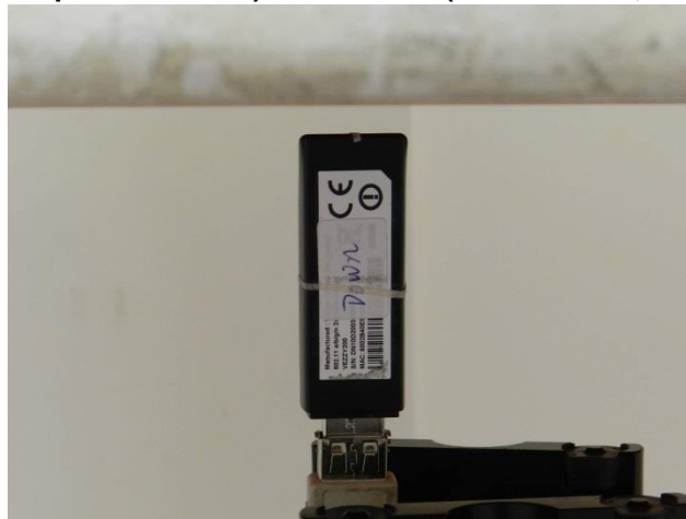
Direct Laptop Plug-in for USB Configuration 5 (Tip Mode, Test Separation 5 mm)
