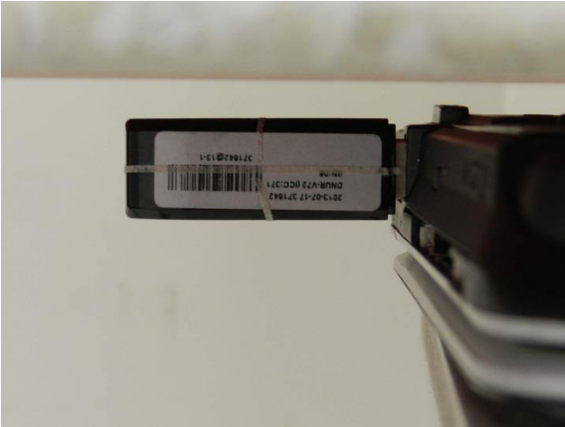
USB Cable Plug-in for USB Configuration 3 (Vertical Front, Test Separation 5 mm)
