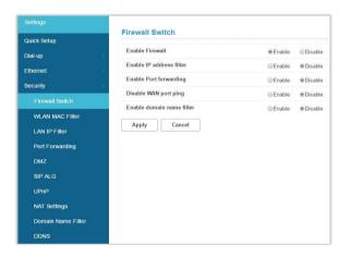
**Enable Firewall:** The Router has a built-in firewall. To disable the firewall, select **Disable**.
