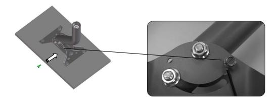
5. Adjust the angle of the pedestal mast. Use the spirit level and confirm the bubble is perfectly located at the center position. Fully tighten the mast screws after confirming the mast angle.
