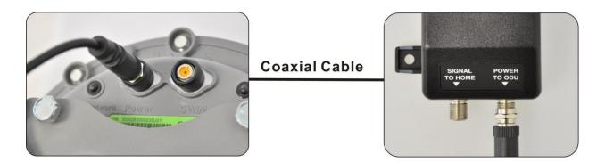
9. Connect a coaxial cable from the **SIGNAL TO HOME** port of the power inserter to your home service gateway.
