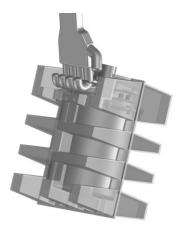
7. Attach the Cantenna to the pedestal and remove the protection pulp. Tighten the 2 bolts on the mounting plate.
