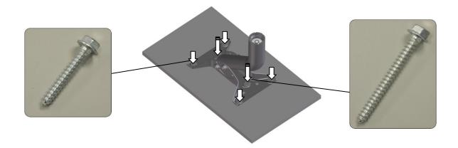
4. Tighten the grounding screw and securely ground the wire.
