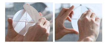
Step 4. To eliminate air bubbles use both thumbs to press in all areas where the Gecko adhesive pad contacts the glass. Press for one minute (30 seconds on the upper part and 30 seconds on the lower part).
