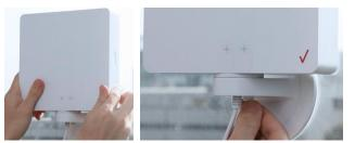
Step 7. Press the scan button to confirm signal.
