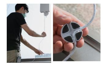
Step 9. Use cable clips and cable spooler to organize cables.
