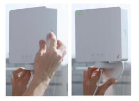
Step 11. Once the LED turns solid green, use the label to mark the installation location.
