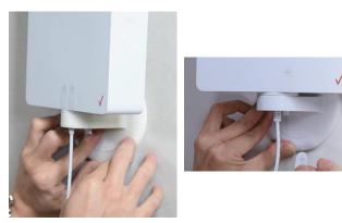
Step 2. Remove the bracket base cover.
