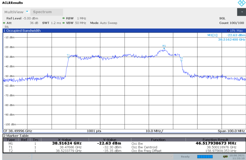
Plot 7-43. Occupied Bandwidth Plot - (n260 50MHz - 16QAM - Mid Channel) – Donor Side – V Beam
