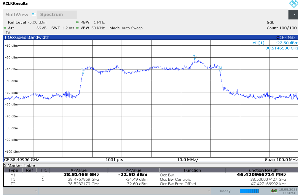
Plot 7-41. Occupied Bandwidth Plot - (n260 50MHz - \pi/2 BPSK - Mid Channel) – Donor Side – V Beam
