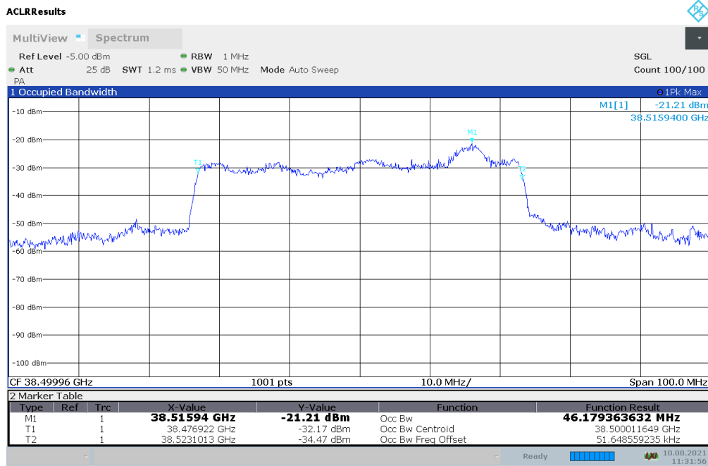
Plot 7-41. Occupied Bandwidth Plot - (n260 50MHz - \pi/2 BPSK - Mid Channel) – Donor Side – V Beam
