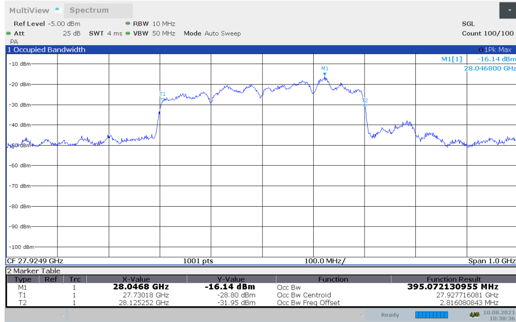
Plot 7-7. Occupied Bandwidth Plot - (n261 100MHz - 16QAM - Mid Channel) – Donor Side – H Beam
