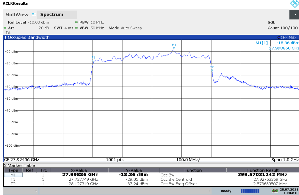
Plot 7-13. Occupied Bandwidth Plot - (n261 100MHz - \pi/2 BPSK - Mid Channel) – Donor Side – V Beam
