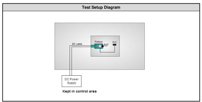
Note: The support notebook was disconnected from EUT and removed from test table when EUT is set to transmit continuously.
