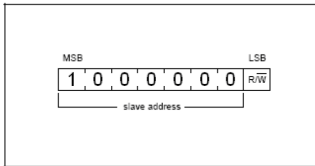
Figure 5: First Byte after the START Procedure
