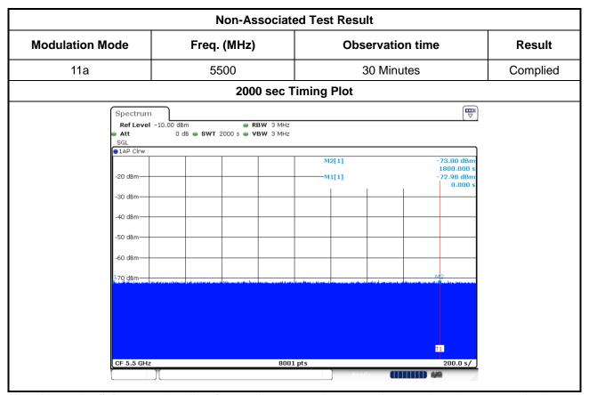
Note: Master is off. Power up the client for 30 minutes to make sure no beacons have been transmitted.
