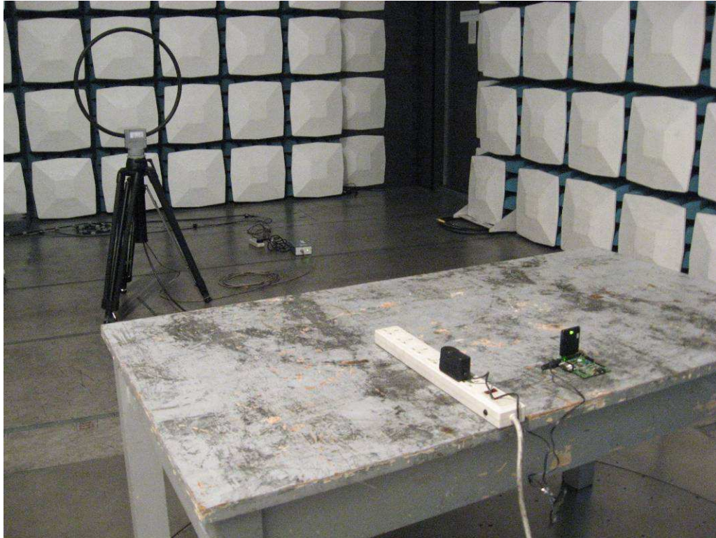
Photograph 4: Set-up for Spurious Emissions (30MHz-1GHz)
