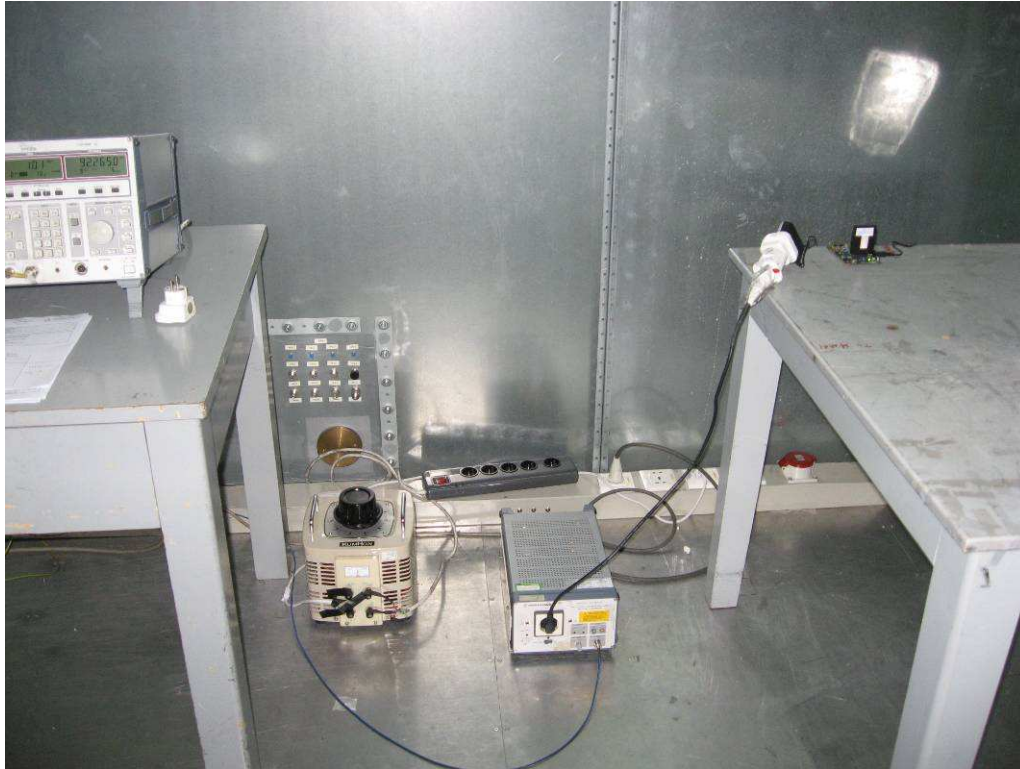
Photograph 7: Set-up for Conducted Emissions
