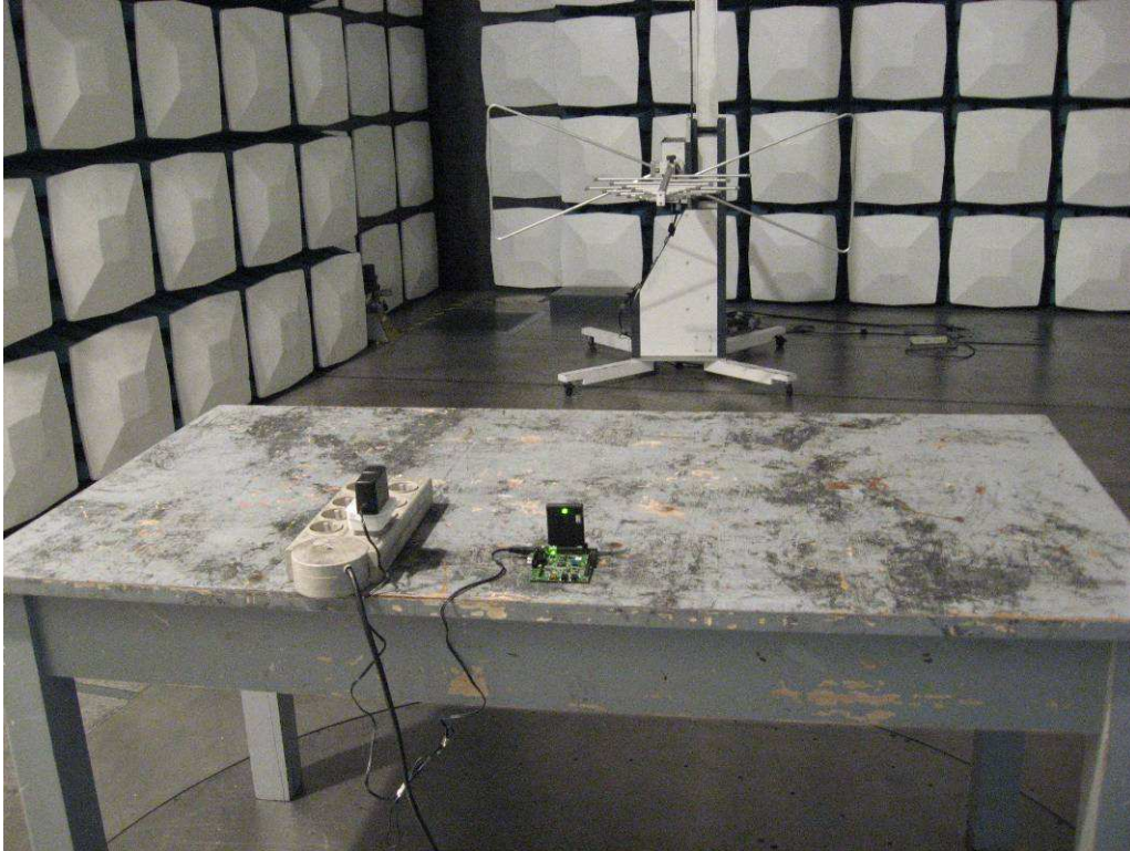
Photograph 2: Set-up for Transmitter test
