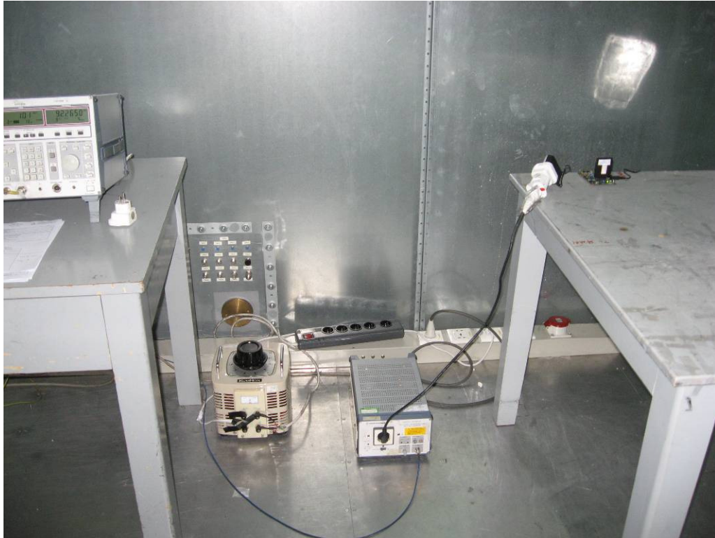
Photograph 7: Set-up for Conducted Emissions
