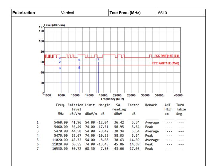
Note 1: ">20dB" means spurious emission levels that exceed the level of 20 dB below the applicable limit. Note 2: For restricted bands, the peak measurement is fully sufficient, as the max field strength as measured
