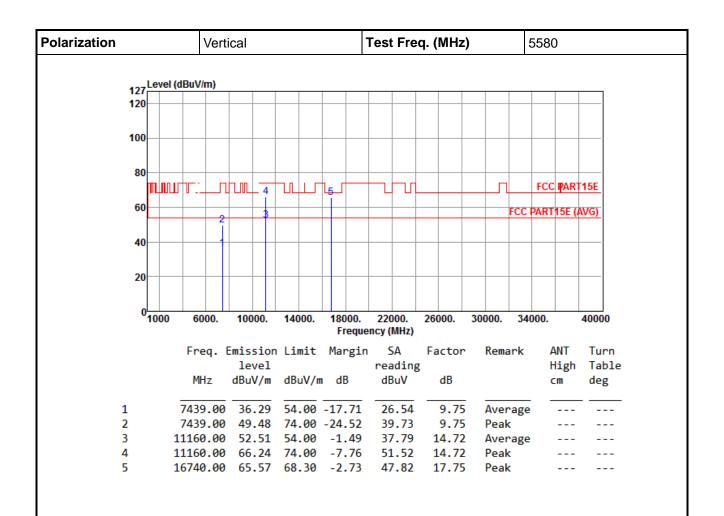
Note 1: ">20dB" means spurious emission levels that exceed the level of 20 dB below the applicable limit. Note 2: For restricted bands, the peak measurement is fully sufficient, as the max field strength as measured
