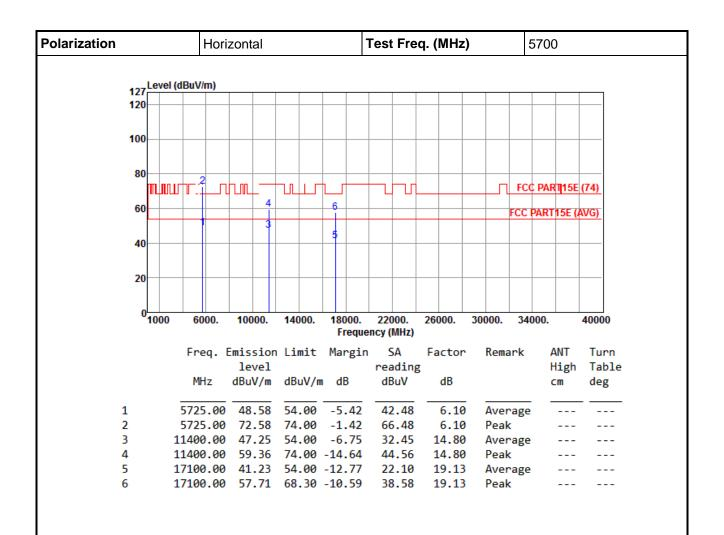
Note 1: ">20dB" means spurious emission levels that exceed the level of 20 dB below the applicable limit. Note 2: For restricted bands, the peak measurement is fully sufficient, as the max field strength as measured
