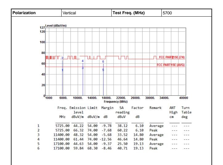
Note 1: ">20dB" means spurious emission levels that exceed the level of 20 dB below the applicable limit. Note 2: For restricted bands, the peak measurement is fully sufficient, as the max field strength as measurement.
