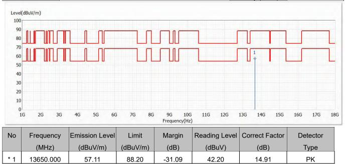
1. All reading above 1GHz is performed with peak and/or average measurements as necessary.
