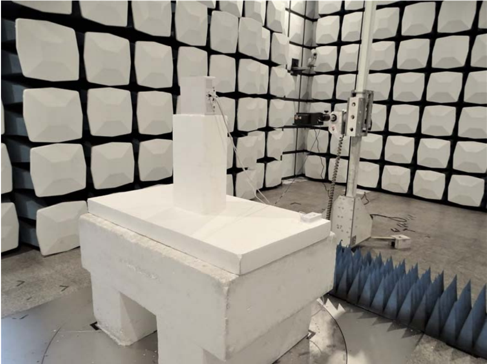
Front View of Radiated Test (Horn) _ 50-200GHz (1m)
