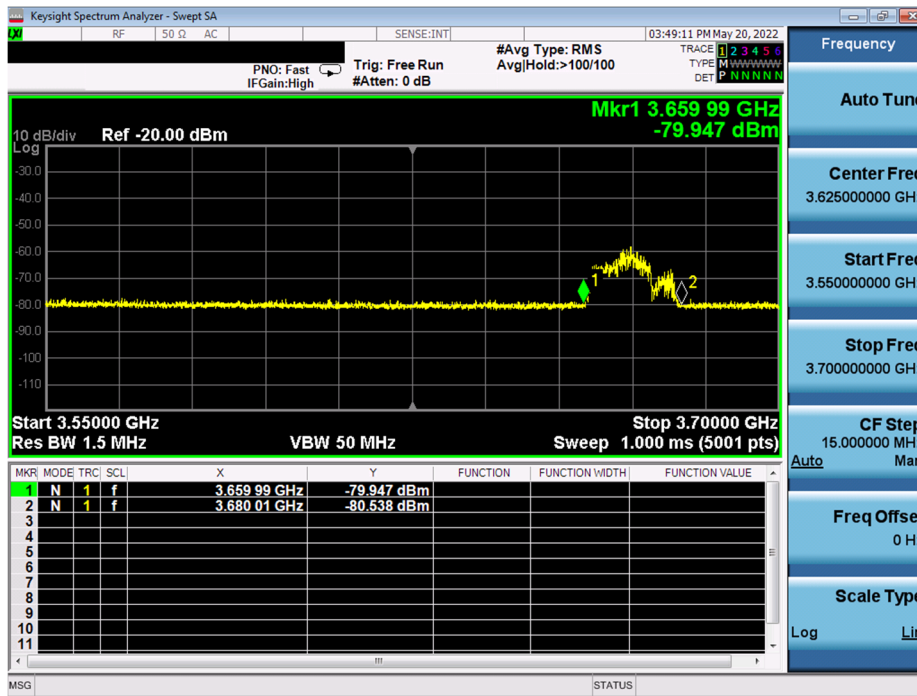
Plot 6-3. Run#2 End User Device Frequency of Operations (3670MHz)
