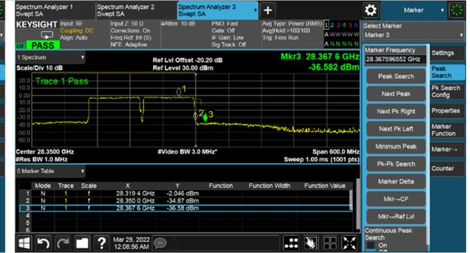
Highest Band edge: n261-BW:100MHz-2CC-QPSK-Beam ID 343
