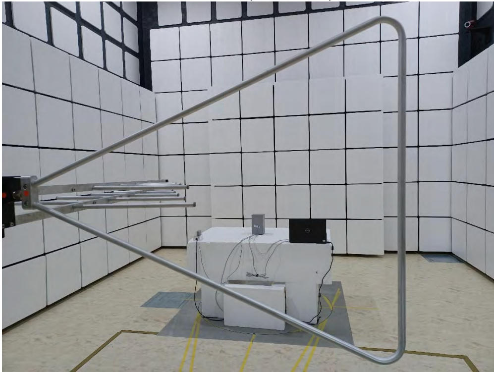
Radiated Test (1GHz to 18GHz)
