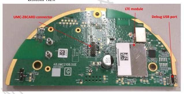
Make sure to connect the Zigbee card
