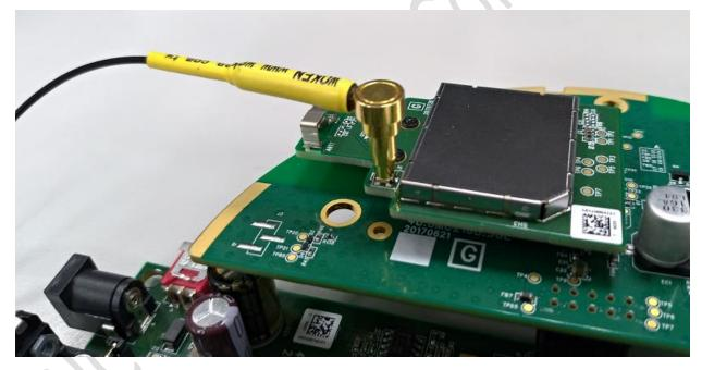
Connect to Zigbee RF connector for conducted test
