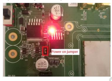
Step3: Press the button of power switch to enable module
