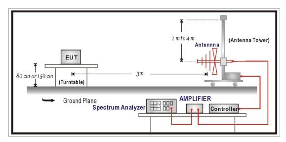
Radiated Emission 1 GHz to 40 GHz-Field strength method
