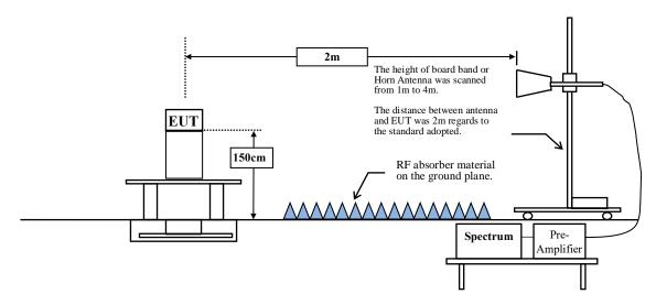
Radiated Emission 50 GHz to 200 GHz-Field strength method
