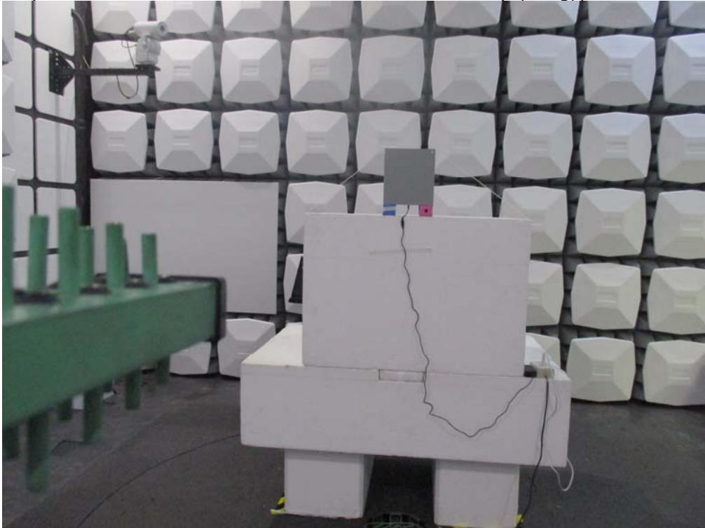
Description : Back View of Radiated Emission Test Setup (Bilog)(ADP-65JH HB)
