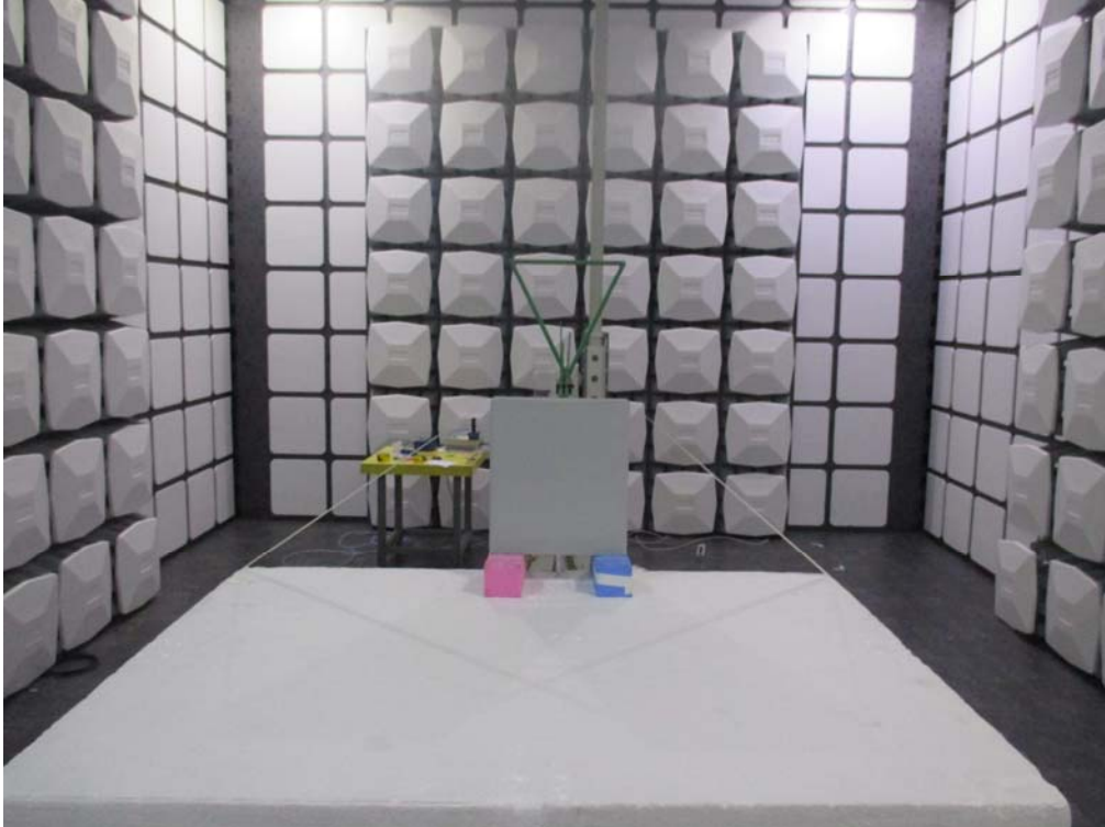
Description : Back View of Radiated Emission Test Setup (Bilog)(ADP-65JH HB)
