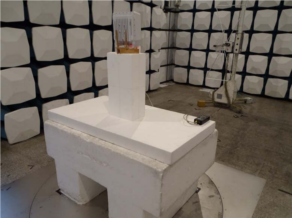
Front View of Radiated Test 30MHz-1GHz (ADH-90AR B)
